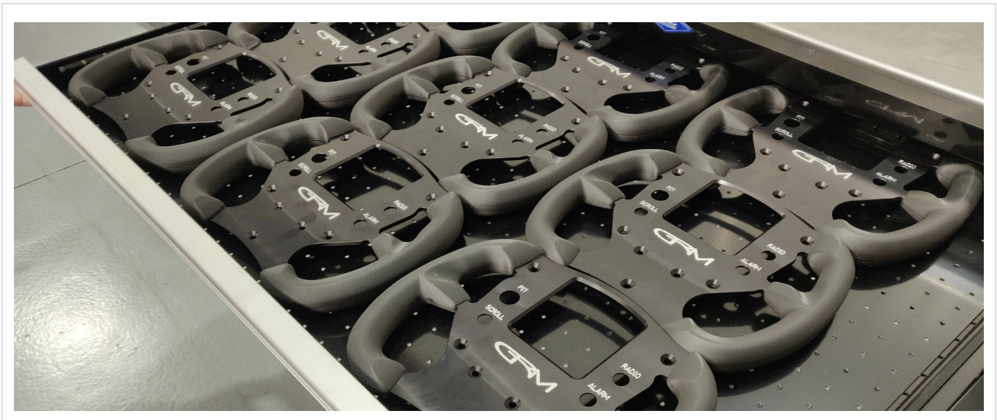
Garry Rogers Motorport used to prototype steering wheels with injection moulded rubber handles, and are now able to 3D print the handles for end use.
