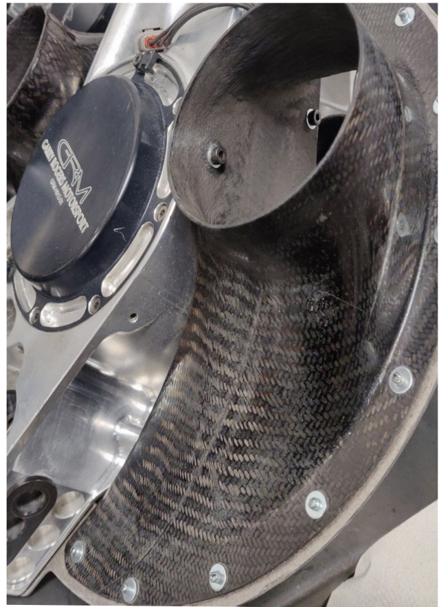
The final brake duct, which was made using a 3D printed brake duct pattern.
