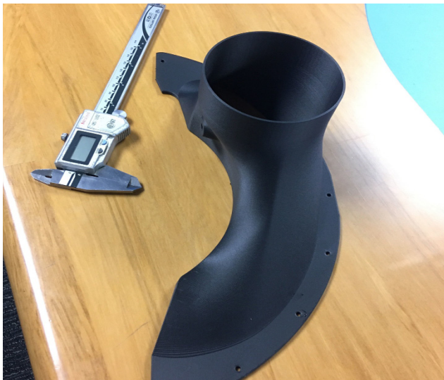
The 3D printed brake duct pattern, printed on the team’s Markforged printer.
