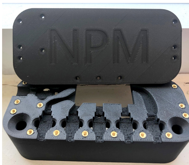
The electronics housing for the Neurophotometrics system takes just under 11 hours to print.
