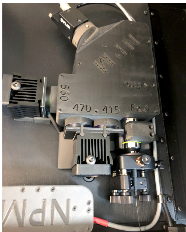
The optical housing and internal components are all 3D printed in Onyx to allow for design flexibility without sacrificing durability.
